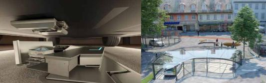
When an electric vehicle with the VOLTERIO charging system approaches to the respective parking lot, the base unit automatically connects to the vehicle's underbody via a powerful physical connection. The VOLTERIO system can be easily retrofitted to almost every electric vehicle.
